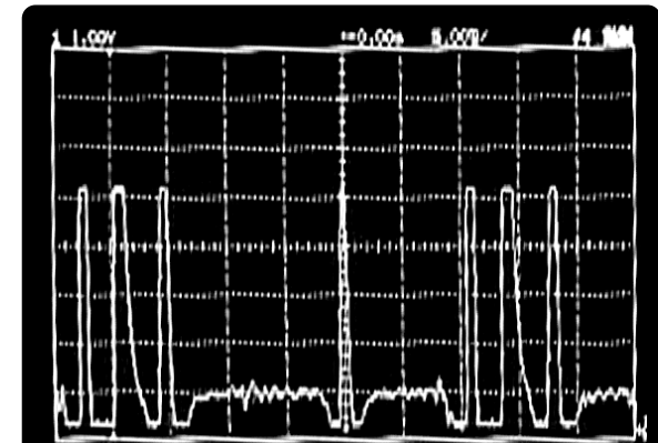
Figure 6.2: Frequency response of several LC tags; distinct “peaks” are visible
